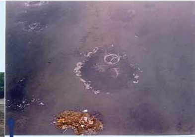
Showing Gas Bubbles indicating Septic Condition in river Musi.
