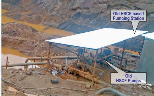
In 2014, for the second stage of pumping (*in first stage, the submersible slurry pumps pumping slurry to the nearby sump*) BAL had purchased 2 Nos. of Aqua's Mine Dewatering Pumpsets for their Thick Slurry (25% by Volume) Water pumping.
