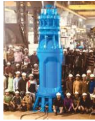
Submerged Turbine Pumpsets (AVT)
