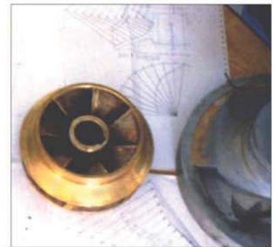
Pattern development of an impeller
