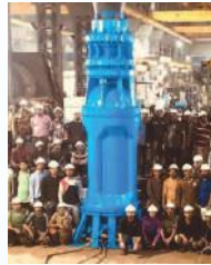
Submerged Turbine Pumpsets (AVT)
