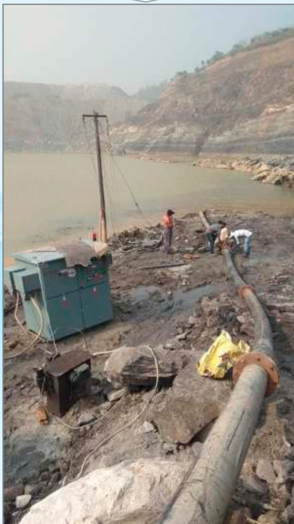
150m x 1835 IGPM, 3.3kV 475hp AMS pumps being used by m/s WCL at Pench (New Sethia OCM)
