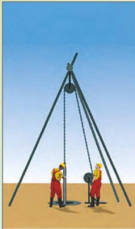
Joining of the Discharge Pipe & Lowering of the Pump to the Proper Setting.
