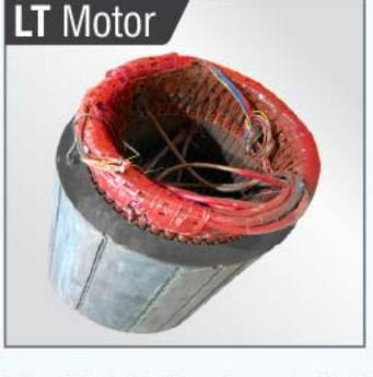
The Totally Enclosed, Self Circulation Water Cooled [TESWC IC-4A1W1 to IEC/IS-60034\_6] motor is similar to Dry Type Induction Motor, the major difference being the Degree of Protection - it is of IP-68 Enclosure to ensure Hermetic Sealing (even if an accidental water flooding the dry-well).
